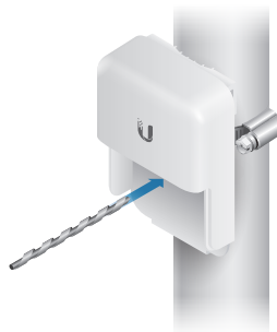
2. Drill a pilot hole into the pole.
